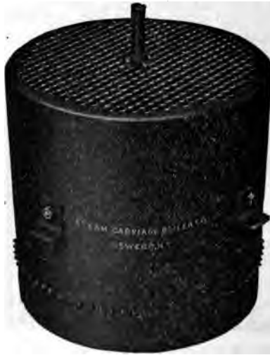
FIG. 335.—Small Carriage Boiler made from a seamless steel pressing, the lower tube plate being flanged over and riveted in, as indicated at the base of the figure, this being the only seam in the structure.
